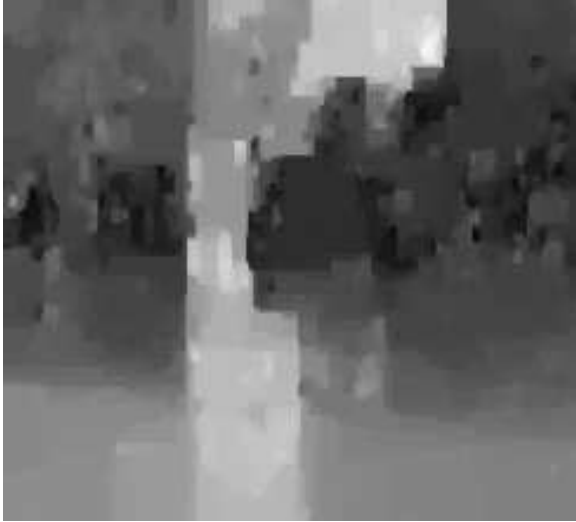
Figure 10: Motion field for SRI Trees presented as depth map. Dark regions are far and light region are close by.
