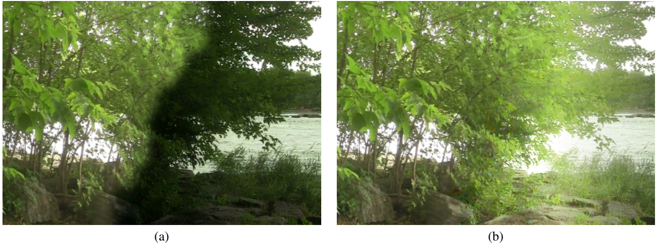
Figure 4. Optimal transition for a single frame within an overlap rendered (a) using the original intensities. (b) after a histogram equalization of the darker block of frames so that it matches the lighter block.
