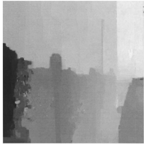
Figure 22. Disparity maps for the Park meter. Results are shown for 4 image sequence. The matching volume is 256 \times 240 \times 64 .
