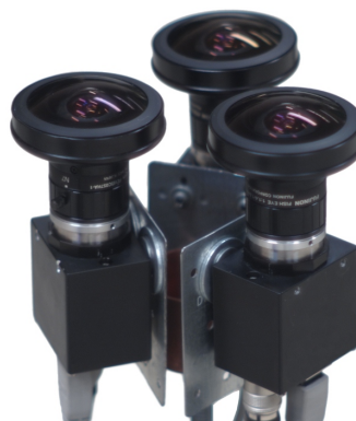
Figure 1. The omnipolar camera setup has no moving parts and is composed of at least 3 cameras with fisheye lens oriented in the same direction.
