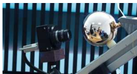
Fig. 15. Home-made catadioptric camera built from a Basler A201bc camera with a Fujinon 12.5mm lens pointed at a Christmas ornament representing a roughly spherical mirror.
