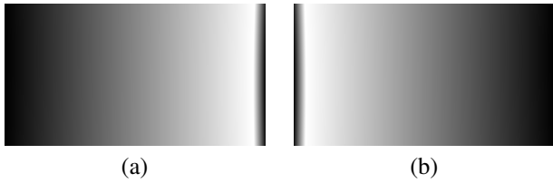
Fig. 7. The blending weight function for the (a) left camera (b) right camera. The function puts more weight near the right or left border instead of the center to minimize the parallax difference between the background and foreground action frames.
