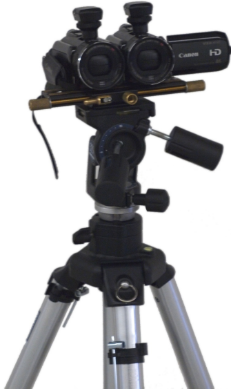
Fig. 11. The setup used in this paper consisted of two cameras in parallel on a tripod. The distance between the projection center of both lens was about 6.5 cm. The cameras were synchronized using the LANC protocol.
