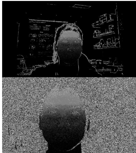
Figure 9. Selected best mix values for a rolling shutter camera. The mix values range from 0 to 1, corresponding to increasing levels of partial exposures between consecutive patterns. The image on the top represents a scan seen by the camera and the image on the bottom by the projector.
