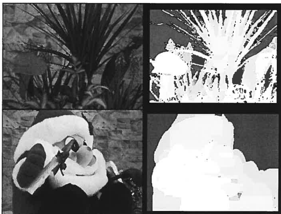
Figure 6.8: Disparity maps for the Plant and Santa scene using DP-Hybrid (Multiview Image Database of the University of Tsukuba). A linear mapping of disparities to gray levels was used.
