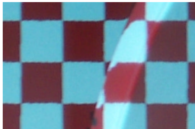
(e) Zoom on errors in the corrected image observed by the camera. The errors are the differences in color between this image and the target image. Black squares (middle bottom) result from holes in the mapping. Distortions are due to interpolation at borders featuring large discontinuities. Intensity variations occur because of varying screen color.
