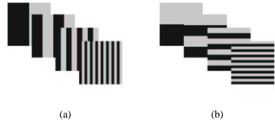
Figure 4. Projection patterns for bits b = 4, 3, 2, 1 . (a) patterns used to obtain R_b^s , (b) patterns used to obtain R_b^t . Inverse patterns are not shown.
