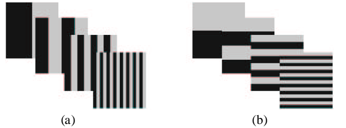
Fig. 2. Projected patterns for bits b = 4, 3, 2, 1 for the s (a) and t (b) coordinate respectively.
