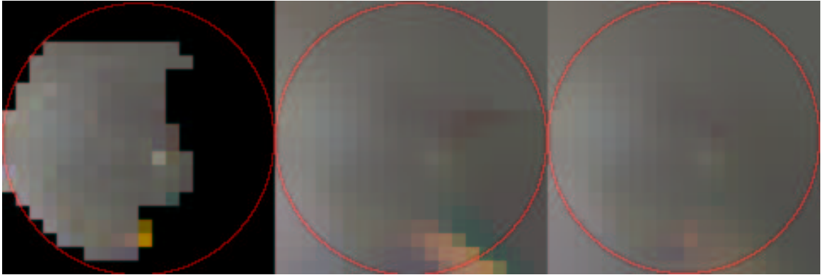
Figure 3.2. Intermediate steps in the processing of a lightsphere. Black represents undefined values and other intensities represent ratios ( intensity = 100 * ratio ). The red circle contains the valid values of the lightsphere. On the left, the result of the vote. In the middle, the lightsphere after weighted averaging. We notice the discontinuity caused by pseudo nearest neighbor extrapolation (near the lower right corner). On the right, the values initially undefined (the black pixels in the left image) are smoothed.
