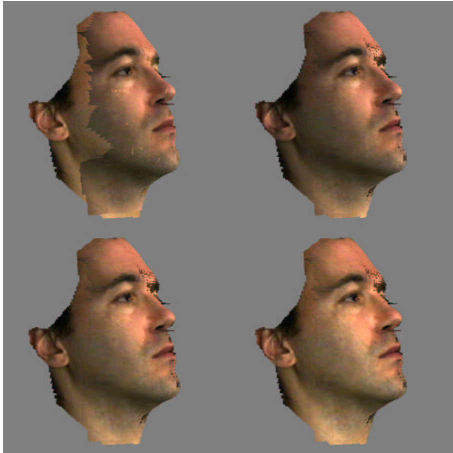
Figure 3.6. Interpolating the illumination. The textures shown are texture-1 on the left, and texture-2 on the right. In the usual order: the original image, the results for B' = B_2 , B' = (B_1 + B_2)/2 and B' = B_1 . The dark spots on the right of each face are not errors, simply the third texture (not modified here).
